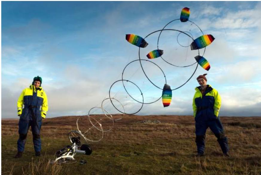
**Fig. 21.13** Rotary ring kite stack in operation, generating  $P_{\text{net}} = 600$  W, showing the portable tracking ground station, the new ring configuration and the force scale (1 December 2017)
