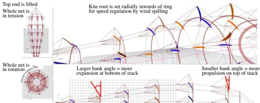
**Fig. 21.10** Driver kites at higher ring levels are set flatter, with a smaller bank angle, and fly faster for overall net dynamic
