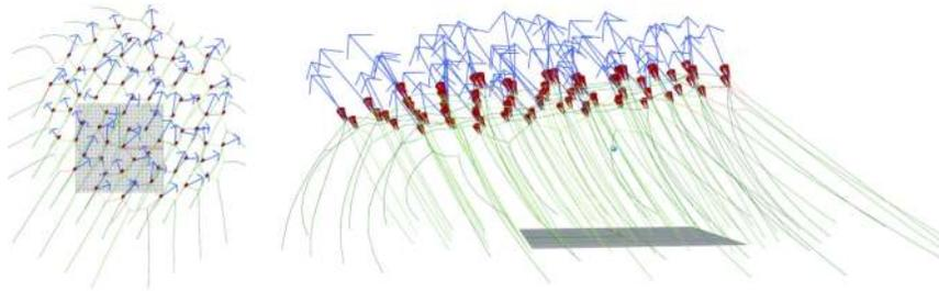
**Fig. 21.11** Model representation of a lifting isotropic network kite (LINK). The resultant aerodynamic force vectors from turbulent wind acting on the individual lifting kites are displayed as blue arrows. Line tension varies from high (red) to low (green). The central lifting lines are held apart and aligned to the average downwind direction despite the action of turbulence on the individual kites
