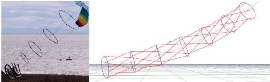
**Fig. 21.8** Ring-to-ring transmission of rotational power employs multiple tethers forming a tensile tubular drive train. Power transmission is smooth despite of the misalignment of the crank at the ground to the lift-normal plane in this prototype and model. Also this setup makes use of a central guiding lifting line
